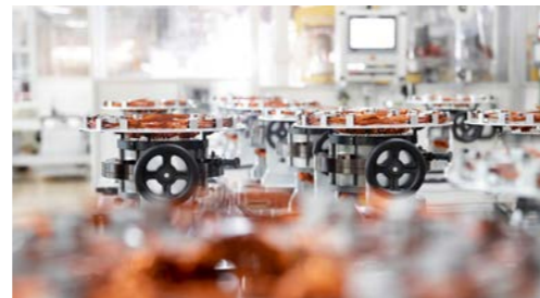
Fully automatic production line for the manufacture of stators with the use of round wire.
