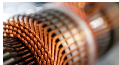
The flat wire wave winding technique is characterized by very few welding points in the wire run. As a result, the manufacturing process is both fast, efficient and reliable in production.
